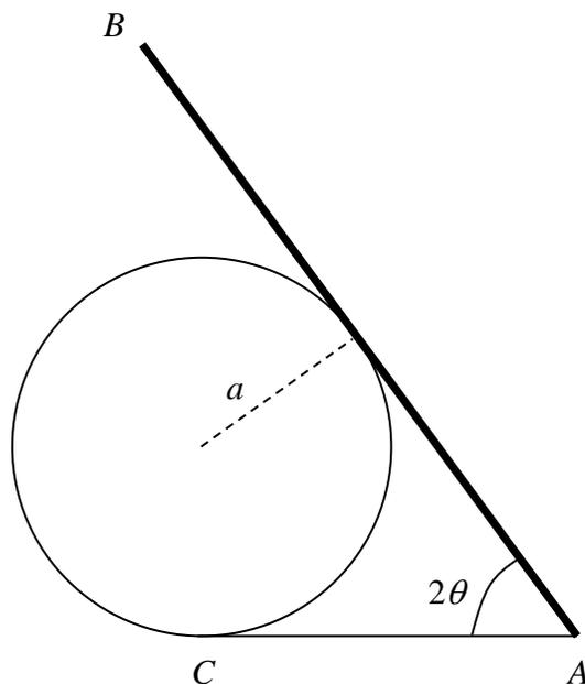
Figure 1 shows a uniform rod  $AB$ , of mass  $m$  and length  $4a$ , resting on a smooth fixed sphere of radius  $a$ . A light elastic string, of natural length  $a$  and modulus of elasticity  $\frac{3}{4}mg$ , has one end attached to the lowest point  $C$  of the sphere and the other end attached to  $A$ . The points  $A$ ,  $B$  and  $C$  lie in a vertical plane with  $\angle BAC = 2\theta$ , where  $\theta < \frac{\pi}{4}$ .
